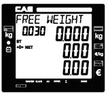
® Remove all weights from platter if user does not need tare function. At this time the weight shows negative value of tare.
